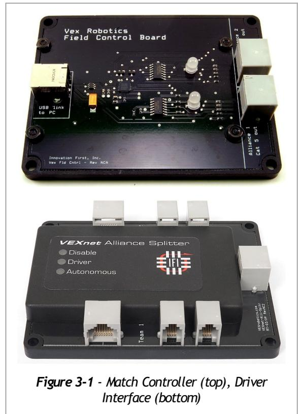
**Figure 3-1 - Match Controller (top), Driver Interface (bottom)**
